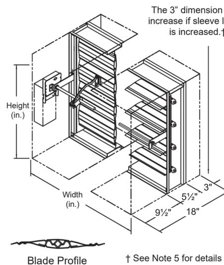
**Smoke Damper ▲ Leakage Class II ▲ Airfoil Blades ▲ 250°F or 350°F Rated ▲ Galvanized Steel**
